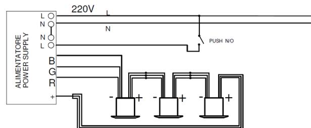
The synchronization is possible with the equipped cable, max 20 devices.
